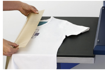
3 Make sure to apply the elements from the recommended side and use the correct pressing aid. To protect the heating surfaces from any glue residue, it is best to cover them with Teflon® film.
