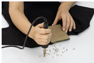
2 Heat the applicator to a suitable temperature and pick up the crystal.
