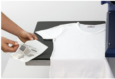
1 Peel off the white protective film*.
