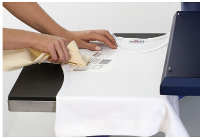
5 After the application is finished, use a pressing cloth to apply additional pressure to the product.
