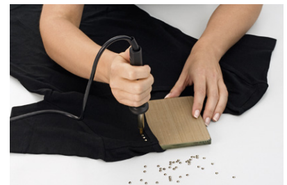
3 As soon as the Hotfix adhesive on the rear of the crystal has melted, position the element on the carrier material, which should be resting on a solid base (e.g. glass, metal).
