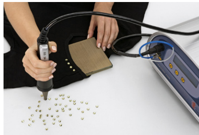
2 Position the crystal on the carrier material, which should be resting on a solid base (e.g. glass, metal).
