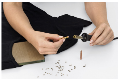
1 Choose an applicator point to match the size of the crystal, so that the crystal cannot tilt out of place or use a plain applicator point.
