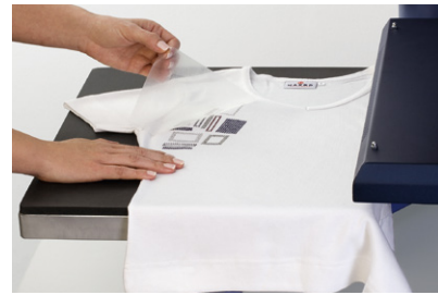
6 Once the product is at least hand warm, the transparent film can be removed at an acute angle.
