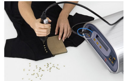
3 Press the adapter firmly onto the crystal at a perpendicular angle and activate the device.
